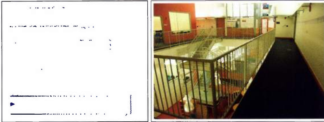
Figure A-8: Partially transparent surfaces. Inferring the correct geometry of a scene is complicated by partially transparent surfaces. Left: the laser data can partially see through the guard rail, detecting both the guard rail and wall on the opposite side. Right: a camera's view of the same environment.
