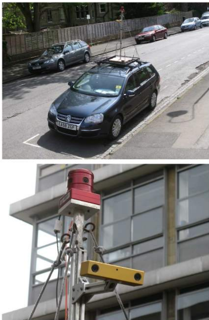
Figure A.2: Vehicle and sensor rig used to capture the 70 km and 1,000 km data sets used in Chapter 5.
