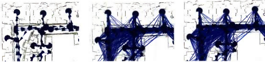
Figure 1-5: Map Building Example. Given the robot’s trajectory (left), we must first identify loop closures (middle). Finally, the maximum likelihood positions of all the nodes, given the loop closures and the original trajectory, are computed (right). The result is a map that is much better than the map resulting from dead-reckoning.
