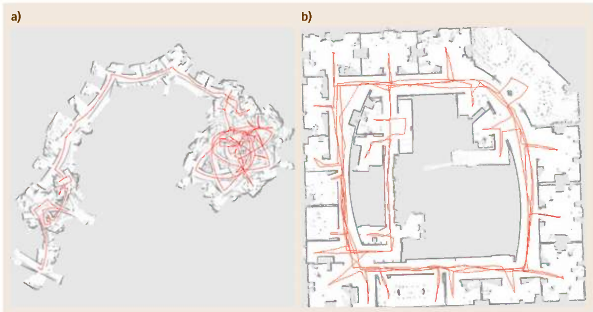
Fig. 46.5 Occupancy grid map generated from laser range data and based on pure odometry (image courtesy of Dirk Hähnel, University of Freiburg)
