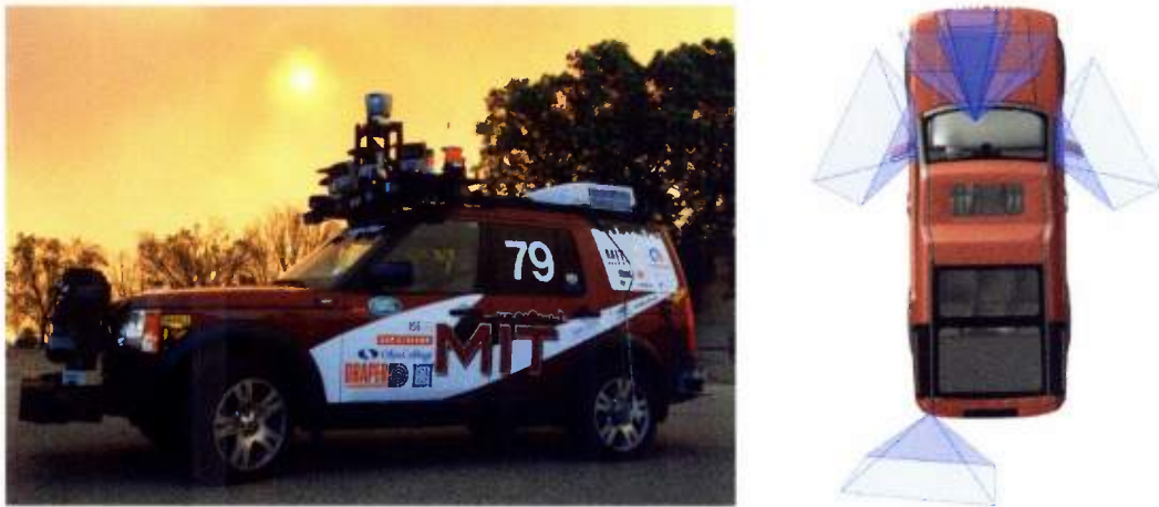
Figure A-1: Talos. Our vision test-bed was MIT’s DARPA Grand Challenge vehicle. The vehicle has five cameras (two forward, left, right, rear), and a high-quality IMU/GPS system for both dead-reckoning and ground-truthing.
