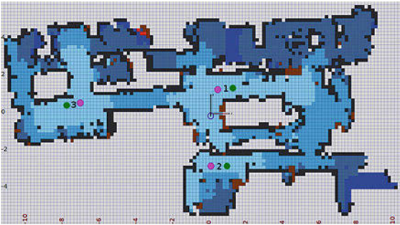
Fig. 65.18 Robot map obtained with vector field SLAM in a 125 m 2 home environment
