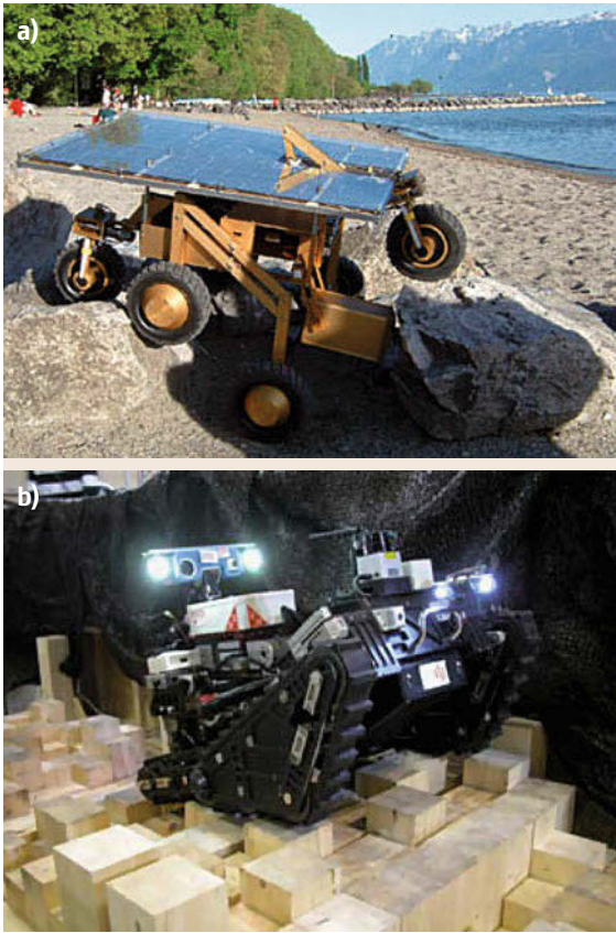
Fig.58.26a,b Mobile platforms with passive adaptation: (a) Solero (after [58.60]) and (b) Robhaz-dt3
