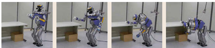
Fig. 67.38 Dynamic multicontact motion generated through global trajectory optimization (after [67.111], VIDEO 597)
