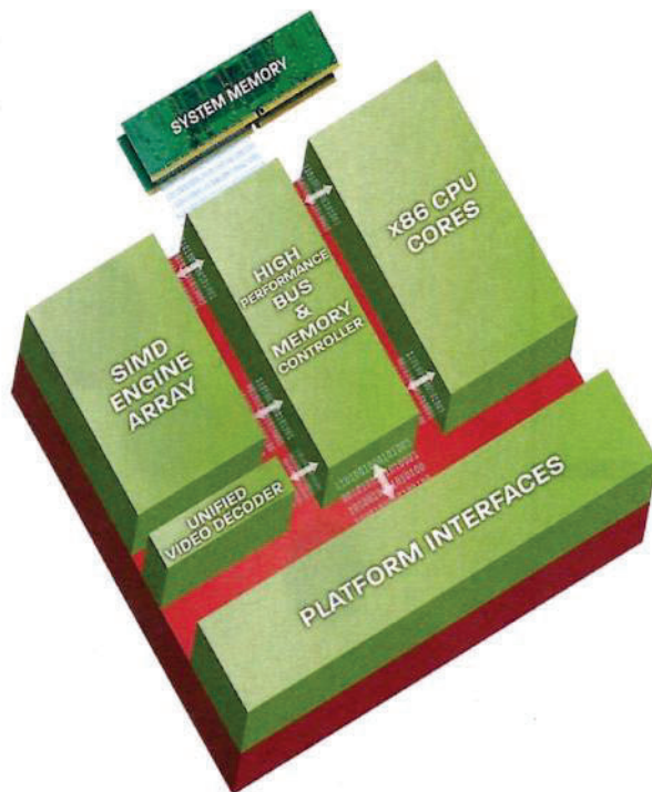
Illustration 10: AMD Fusion Architecture
