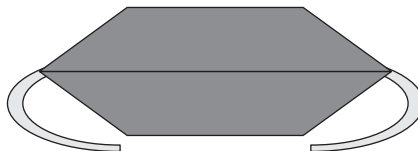
Figure 2.1 J-lead leaded plastic package (not to scale).
