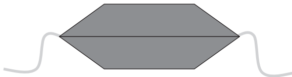
Figure 2.2 Gull-wing leaded plastic package (not to scale).
