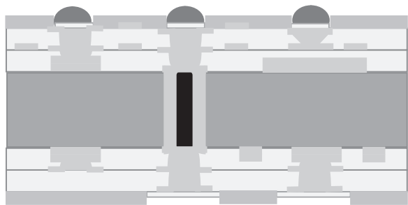
Figure 6.26 Cross section of a 2-2-2 buildup substrate (not to scale).
