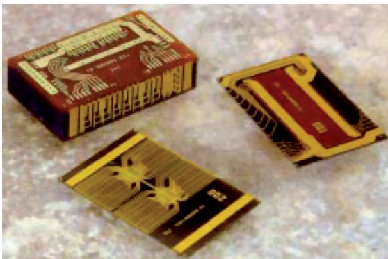
Figure 1.8 Flash neo-stack and its composite layers.
