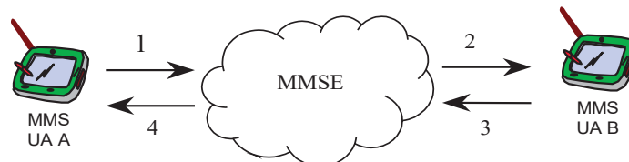
Figure E.1: Message flow in case of reply-charging
