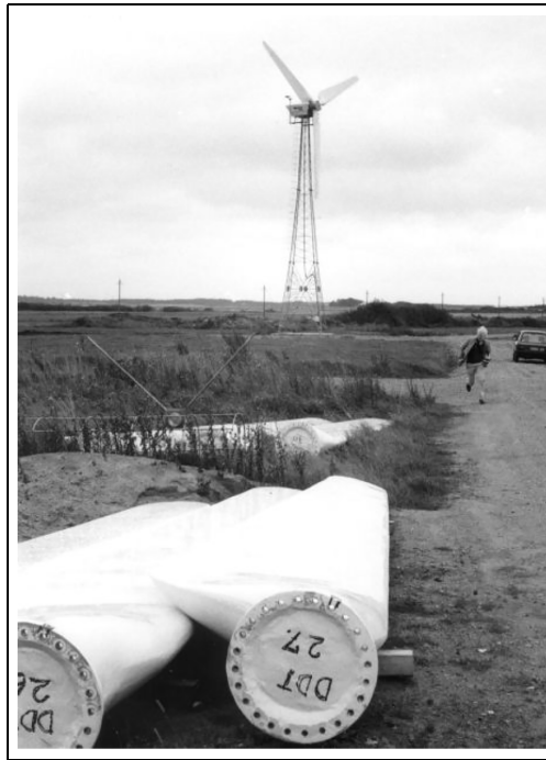
Figure 18. Vestas wind turbine and Økær blades. Background. An HVK wind turbine in Vestas livery at the Vestas plant in Lem. Vestas bought the turbine and design from HVK before launching its successful line of 15-m diameter wind turbines. Foreground. Økær 7.5-m blades with pitchable blade tips developed by pioneering Danish blade designer Erik Grove-Nielsen. Note the “Hütter flange” that made it all work. 1980.
