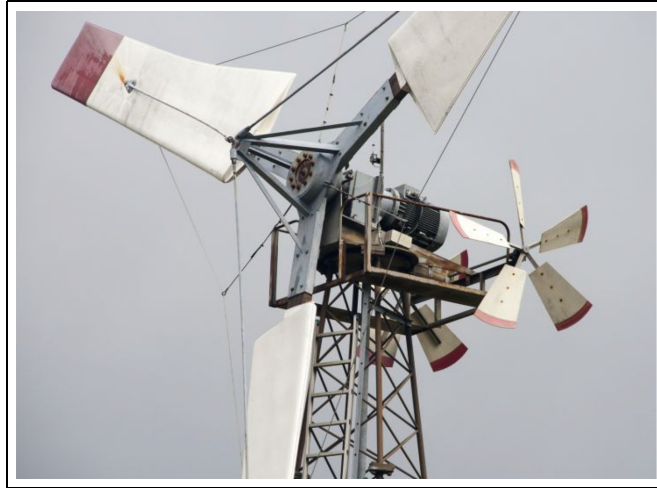
Figure 11. Riisager: One of the pioneering Danish wind turbines during the great wind revival of the 1970s and early 1980s. Laminated wood blades, struts and stays reminiscent of Juul's Gedser mill, and fantails for orientation from the la Cour tradition are all found on this 30 kW version of Christian Riisager's turbine at the Energmuseet , the Danish Museum of Energy near Bjerringbro. Hundreds of derivatives of Riisager's design were installed in California and Denmark. Some were still operating in Californian's Altamont Pass in the mid 2010s.
