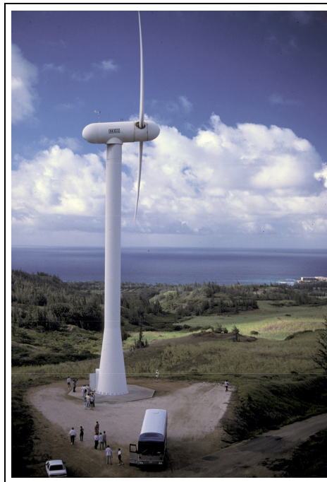
Figure 4. Westinghouse 600. One of the more successful ventures resulting from the US research & development effort was Westinghouse's 600 kW model. Fifteen turbines were installed in Hawaii and operated for a number of years. They were eventually removed and two surviving turbines now stand at the National Renewable Energy Laboratory at Rocky Flats, Colorado. Late 1980s.
