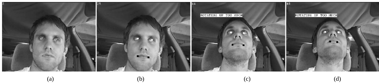
Fig. 17. Driver visual attention output. (a) No messages, (b) rotating up too much, (c) rotating up too much, and (d) rotating up too much.
