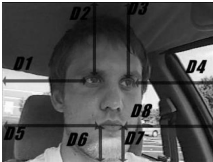
Fig. 8. Distances that the program monitors to classify rotation.
