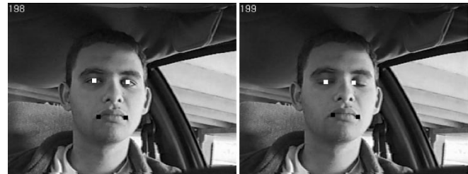
Fig. 6. Feature tracker with eye blinking.
