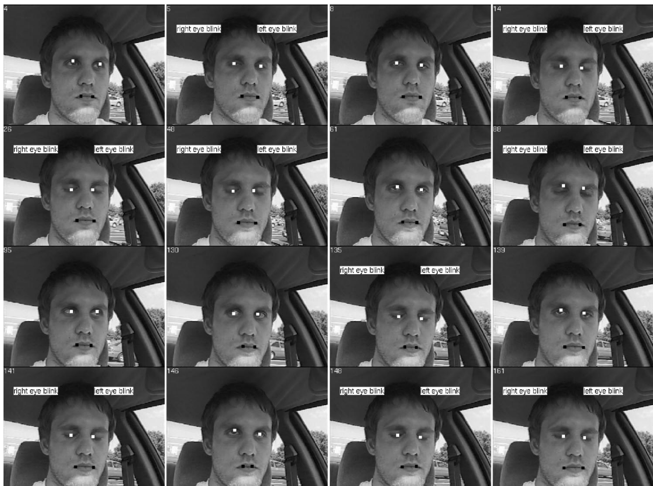
Fig. 20. Blink detection with feature tracker.
