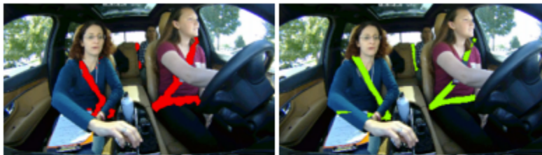
Figure 5: Seat belt detection result ( left ) in comparison with the ground truth ( right ). With human inspection, the prediction result is of good quality as it correctly marks the seat belt area. However, IOU for this particular example was 46%, justifying the need for a better evaluation metric.
