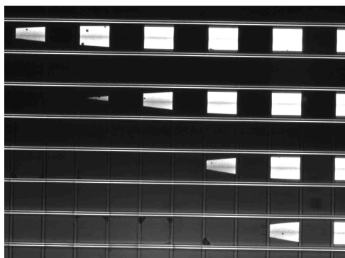
Figure 13: Optical microscope picture of some pixels near the edge of a display aged for 300 h in 60°C/90% RH. Only alternative rows were biased during the measurements.
