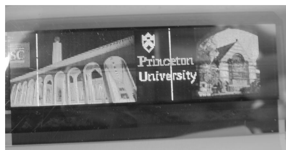
FIG. 3. Thin film encapsulated PHOLED display on 178 \mu\text{m} barrier coated PET. The encapsulation is comprised of five alternating pairs of \text{Al}_2\text{O}_3 and polyacrylate; total thickness of the multilayer barrier stack is 5–7 \mu\text{m} . The 64 \times 240 display is passive matrix and capable of full motion video.
