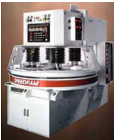
Fig. 20. Schematic of multi wafer per platen polisher [78].
