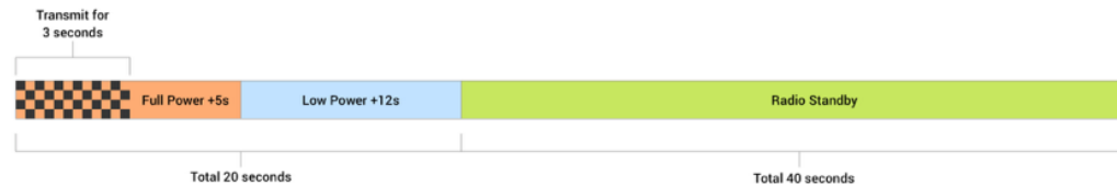
Figure 3. Relative wireless radio power use for three second transfers running once every minute.
