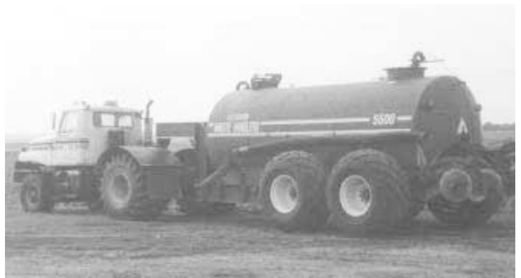
"It lets us go fast and reduces compaction," says Dennis Hess, who converted a "Terra Truck" floater sprayer to pull a big liquid manure tank equipped with injectors.
