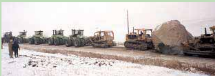
With seven tractors pulling and a D-6 and D-8 pushing from behind (about 3,000 hp in all), they headed down the road - in low gear all around.
