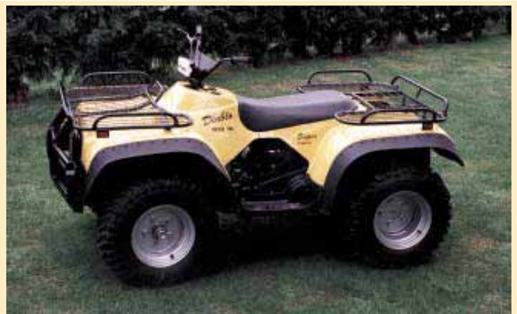
The Diablo, shown above, is powered by a 2-cyl. water-cooled diesel engine.
