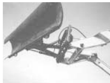
Cylinders on the blade allow it to be angled left or right.
