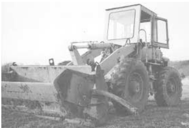
In order to cut through 3-in. dia. phone cable, Walter and Philip Miller added a 2-ft. sq. steel shear plate to the bucket of their IH payloader.
