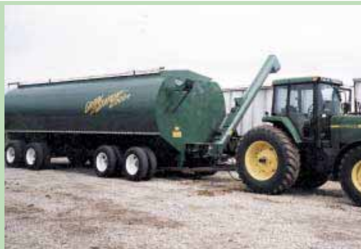
"Grain Station 2000" measures 12 ft. wide and 36 1/2 ft. long. Fully loaded, it holds 61 tons and has 50 percent more capacity than a conventional semi truck.
