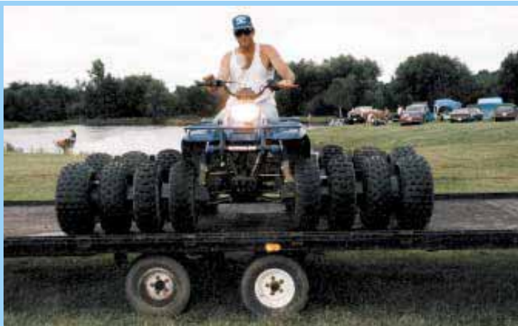
A local metal shop built spacers from rolled pieces of steel to hold wheels on ATV. Riddlestine hauls the big rig sideways on a snowmobile trailer.
