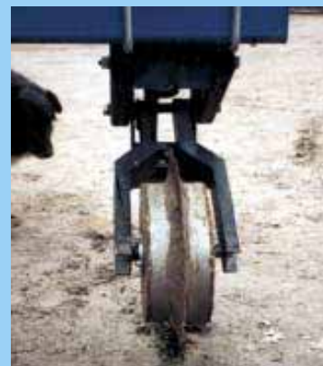
Depth wheels mount on heavy adjustable brackets made from 2 by 4-in. sq. tubing. Plesum says he built the brackets “as heavy as he could”. The wheels are made from a fluted coulters with sections of 12-in. dia. steel tubing welded to either side of it.
