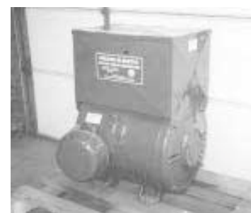
Converter allows you to produce your own 3-phase power from a single phase line.
