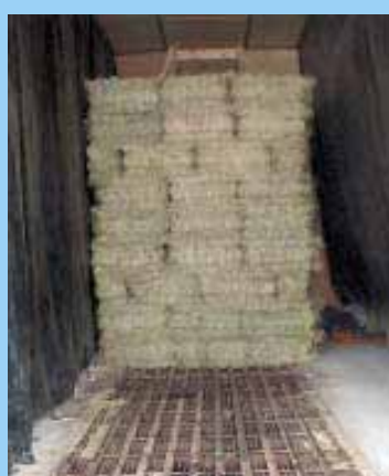
Building houses twin dryers capable of simultaneously drying 800 bales each.
