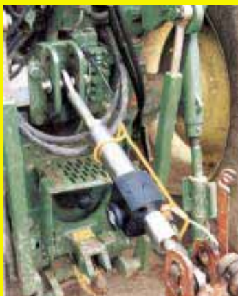
Weigh system does the job of a top link and also weighs whatever is being carried.
