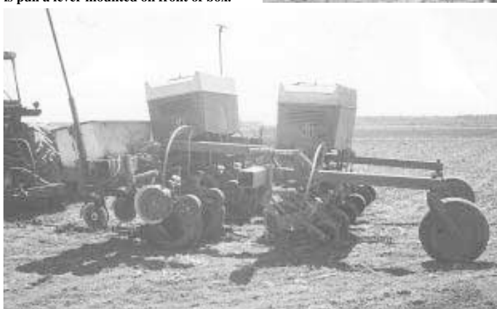
Wallace's twin-row planter is built out of two Case-IH 800 6-row air planters. It plants six sets of twin rows spaced 8 in. apart, with 22 in. between each set of rows.
