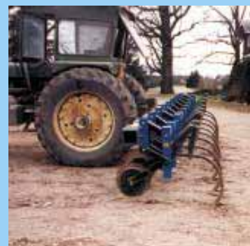
He used conventional Deere chisel shanks fitted with 24-in. wide shovels but built everything else himself.
