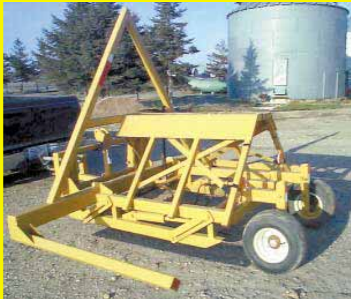
A front-end loader is used to place bales on this "stooker". Side arms lower hydraulically to the ground to unload.
