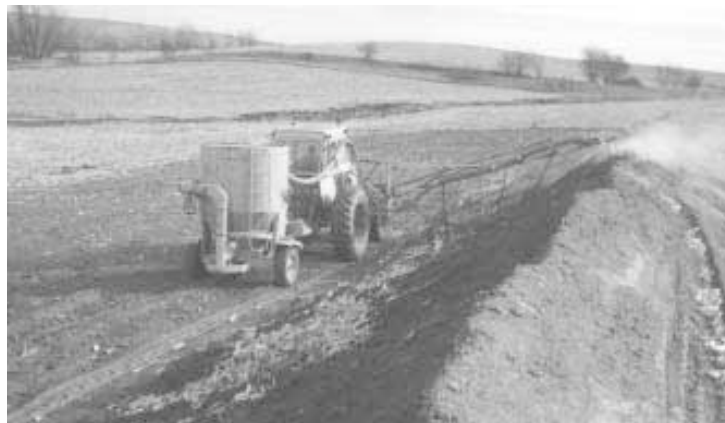
Seed is blown onto side of terrace. Chains that hang from boom cover it with soil.
