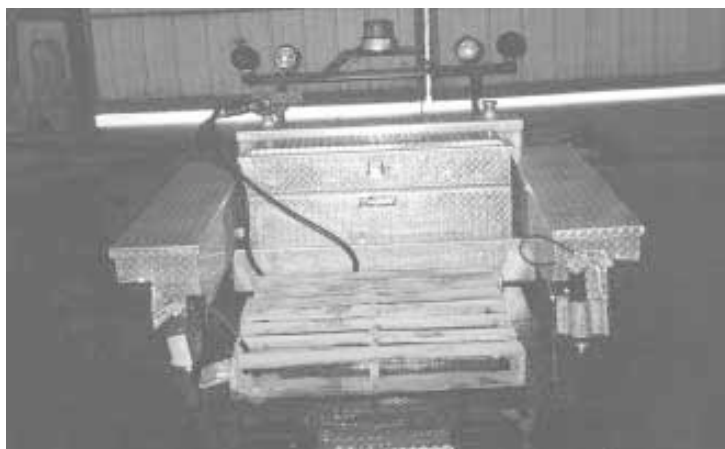
A 90-gal. fuel tank and electric pump topped by a tool chest and light bar mounts at one end of platform, with longer side-mount tool boxes on each side.
