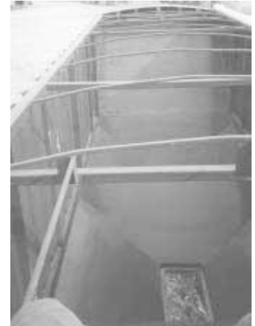
Steve Reinhardt bought pieces of a hopper bottom trailer and welded them together himself, saving thousands of dollars off the price of a finished trailer. Note hopper bottom (right).
