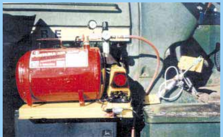
A 5-gal. air tank, 12-volt compressor, 8-in. cylinder, and valve allow Roberts to activate the clutch on his Deere 4430 tractor by either hand or foot with very little effort.
