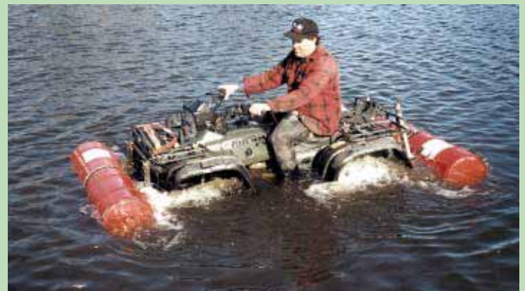
A length of pipe clamps onto exhaust muffler to serve as a “snorkel”. Another snorkel fits the air intake (not shown). The snorkel allows water to wash over ATV.
