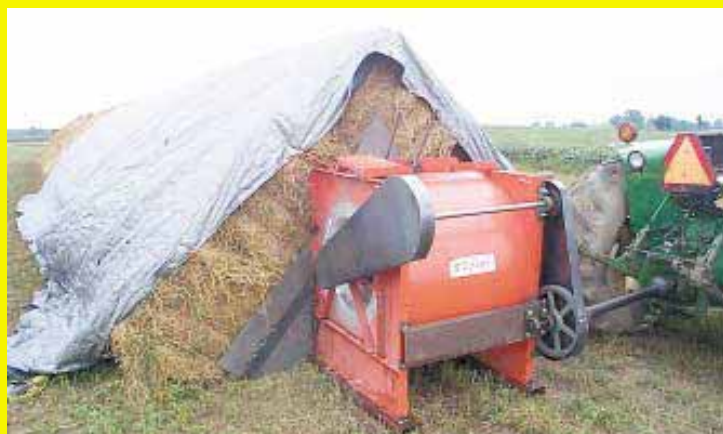
A grain drying fan or silage blower is used to blow air through the tunnel under the bales.
