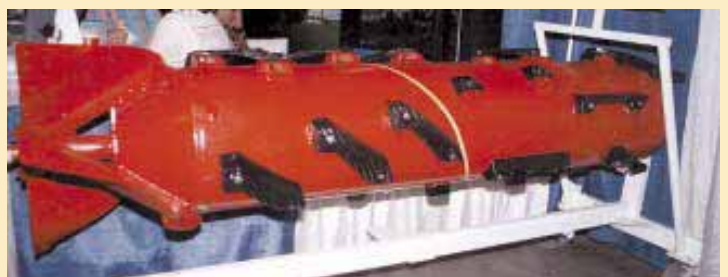
"High-inertia" rotor is actually a rebuilt Case-IH rotor. Kuchar re-attaches the rub bars in a more open design which allows the crop to go through faster without "slugging down" the rotor.
