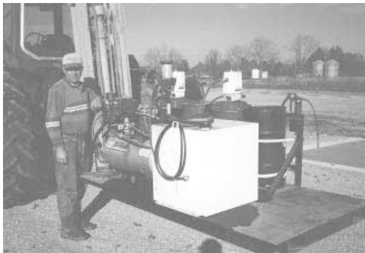
The 4 by 8-ft. metal platform is fitted with a portable air compressor, air-operated grease gun, 50-gal. fuel tank, and three 120-lb. grease drums.
