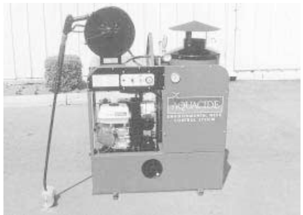
Extreme heat of water immediately destroys the cellular structure in vegetation, killing the plant.
