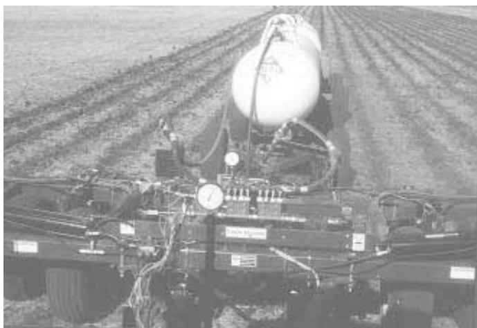
Anhydrous system allows the Harms to evenly apply anhydrous across the width of applicator. Anhydrous is kept in liquid form right down to the knives.
