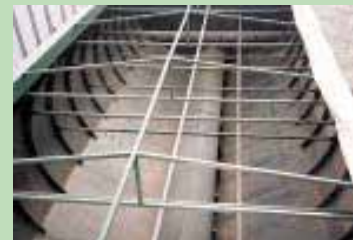
Grain is loaded into an 8-ft. long opening on top and is delivered forward to front unloading auger via a 22-in. wide drag conveyor.
