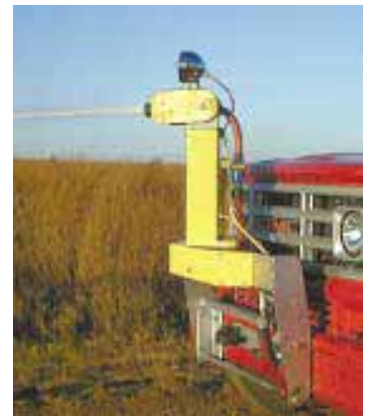
Fire-fighting nozzle mounts on front of pickup bumper and is controlled by a joy stick inside cab. Note spotlight on top of nozzle.
