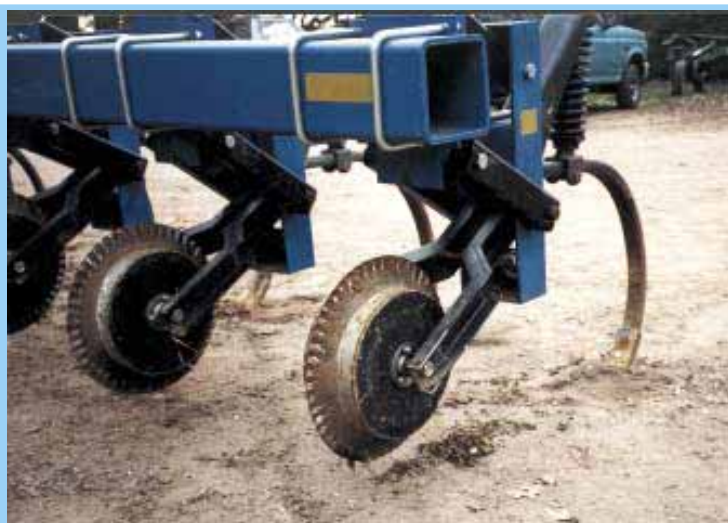
“It’s built heavy and has infinite depth control from 0 to 8 in. deep, thanks to its unique depth control wheels,” says Karl Plesums about his home-built cultivator.
