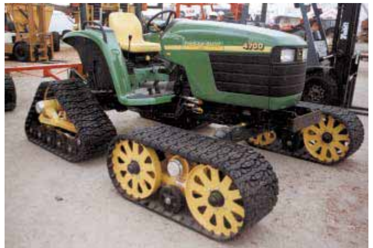
New Mattracks track conversion system is available for smaller 4-WD tractors. It consists of four separate sets of 16-in. wide tracks.
