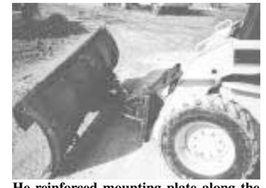
He reinforced mounting plate along the edges and across the center by welding channel iron on back.
