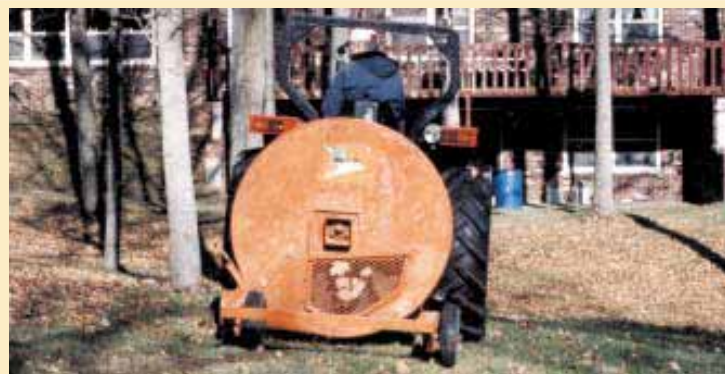
"It has really cut down the time it takes to clean leaves out of our yard," says Pete Lamp about the leaf blower he made out of a pto-driven silage blower.
