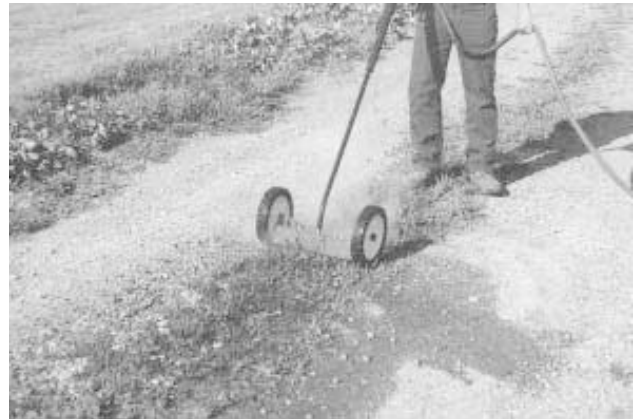
Weeds need to be within 6 in. of nozzle in order to be killed, since heat dissipates quickly into the air.
