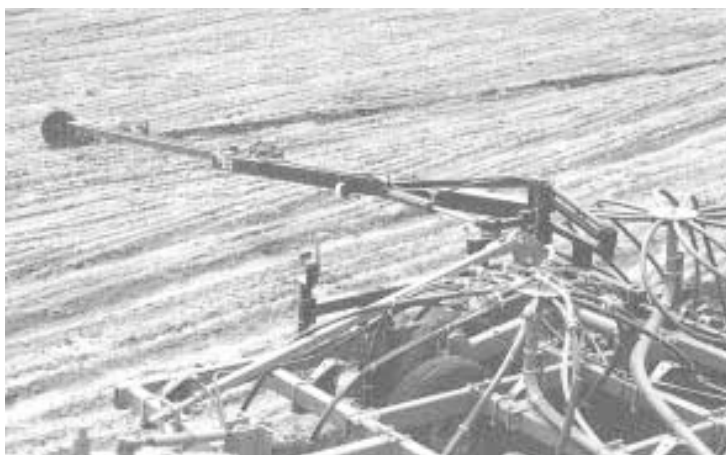
Marker mounts on rear corner of air seeders and cultivators. It swings forward and telescopes to the desired length and leaves a groove of about 2 in. in the ground.
