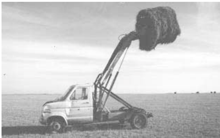
Maxfield stripped off the back of a Ford van and fitted it with a Farmhand F11 loader.
