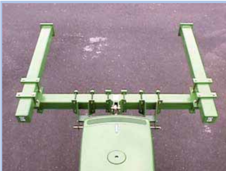
Three-piece toolbar uses one crossbar just ahead of the 3-pt. to support two other bars, which extend forward to clamp onto cultivator toolbar.
