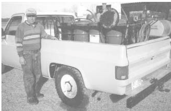
Slide-in "service bed" fits snugly between the wheel wells of Colson's pickup.
