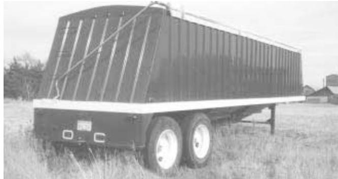
Trailer mounts on axles from an old oil tanker trailer, which Reinhardt rebuilt. He uses a semi tractor to pull the unit.
