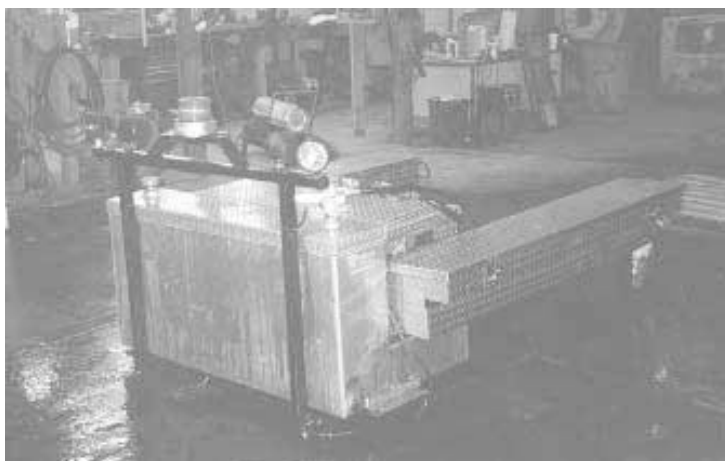
"Tool pallet" is a self-contained shop-on-wheels that slips into pickup with a forklift.
