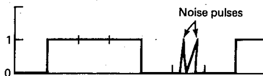
FIGURE 14-17 Data stream with noise pulse.
