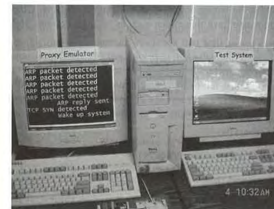
Fig. 14. Photograph of phase 1 (emulator) proxying Ethernet adapter.
