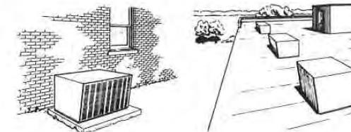
Fig 13-12. Remote condensing unit application
