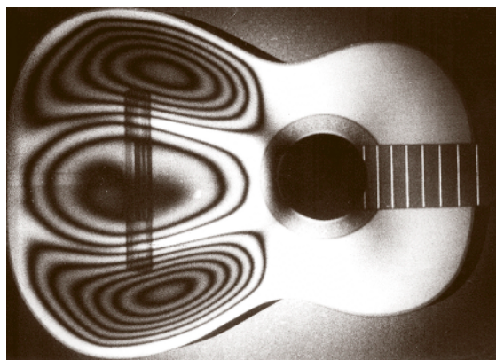
Fig. 27.3 Time-average interferogram of a guitar top plate vibrating at 505 Hz (Bolin guitar from 1969).
