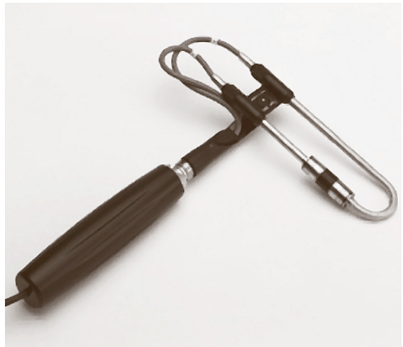
Fig. 25.7 Sound intensity probe with the microphones in the face-to-face configuration (Brüel & Kjær, Denmark)
