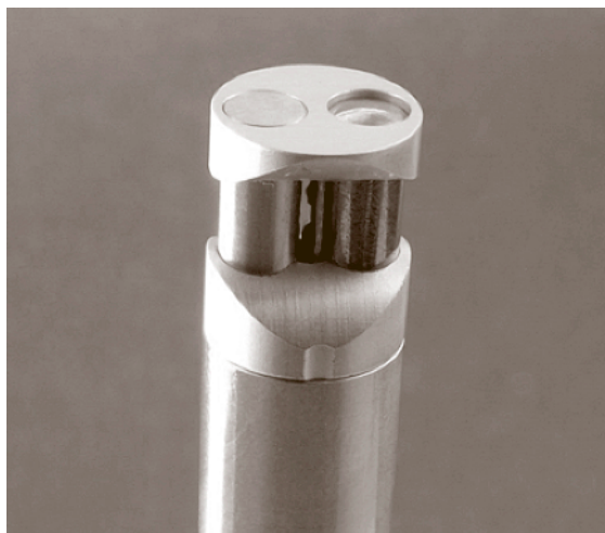
Fig. 25.18 A p - u sound intensity probe (by Microflown Technologies, The Netherlands)
