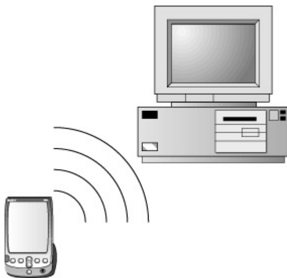
Figure 9.1: A typical IrDA connection
