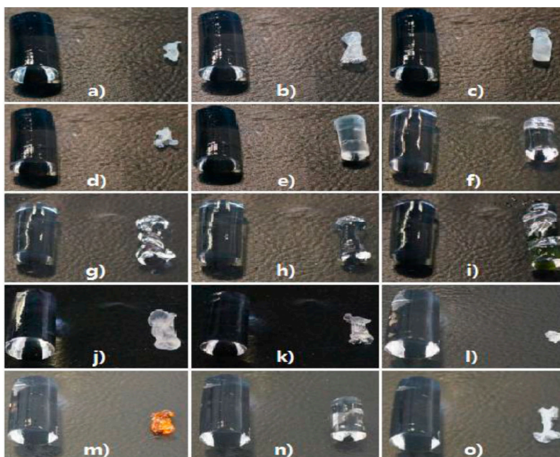
Figure 1. Pictures of shrunk gels compared to an original hydrogel. The hydrogels are placed on the left in each picture, and on the right are the gels once soaked in (a) methyl ethyl ketone (MEK); (b) isopropanol (IPA); (c) acetone; (d) 1-butanol; (e) methanol (MeOH); (f) dimethyl sulfoxide (DMSO); (g) glycerol; (h) propylene glycol; (i) ethylene glycol; (j) ethanol; (k) 1,4-dioxane; (l) propylene carbonate; (m) furfuryl alcohol; (n) N,N -dimethylformamide (DMF) and (o) acetonitrile.
