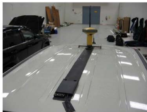
Figure 4-26 Topcon Antenna Mount on Test Vehicle
