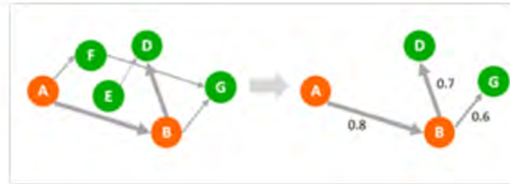
Figure 5: Expansion - aggregate weights and apply threshold
