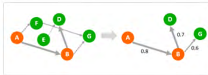
Figure 5: Expansion - aggregate weights and apply threshold
