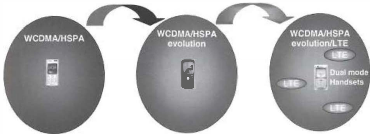
Figure 2.3 One HSPA and LTE deployment strategy: upgrade to HSPA Evolution, then deploy LTE as islands in the WCDMA/HSPA sea.
