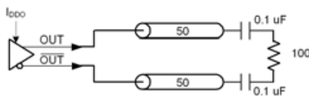
Differential Output Test Configuration
