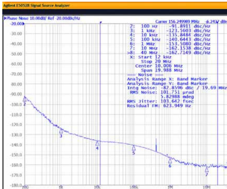
Figure 6. Input = 25 MHz; Output = 156.25 MHz, 2.5 V LVDS
