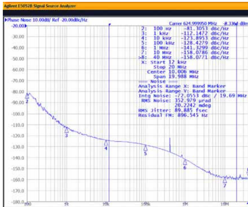
Figure 5. Input = 25 MHz; Output = 625 MHz, 2.5 V LVDS
