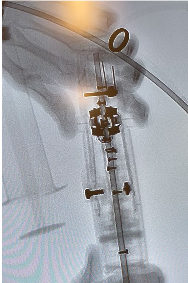
(X-ray image showing button and actuator when button undepressed.)
