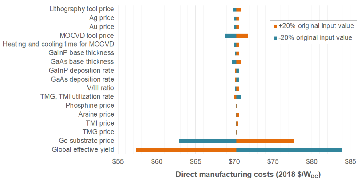
Figure 3. Sensitivity of direct manufacturing costs for the 3J LM III-V solar cell to changes in key input parameters
