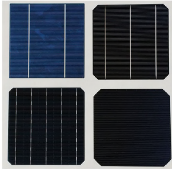
Fig. 9.1 c-Si solar cells with (from the top left) two (2BB), three (3BB), five (5BB) busbar and cell without busbars (below right). Current-collecting fingers are placed perpendicular to the busbars
