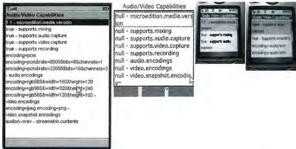
Figure 8-1. MMAPI capabilities in Sun's DefaultColorPhone emulator, Motorola C975 emulator, and Motorola C975 device (last two figures)
