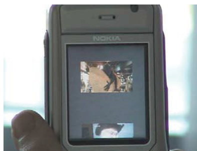
Figure 6: Picture browser application. In this prototype, a large collection of photographs is presented. The user can move their phone to scroll through the collection. If they slow down their movement, the application automatically adjusts the zoom level to help the user browse.
