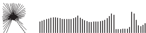
Figure 6: An example of extracting the centroid-to-boundary distances for the character 'R'.
