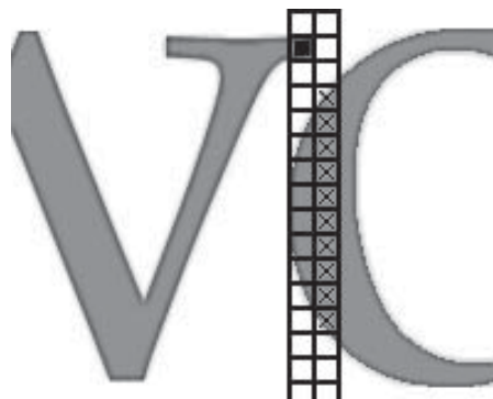
Figure 4: Distinguishing two characters from each other. The all-black square is a pixel that belongs to the connected component that comprises the current character. Since none of the pixels belonging to the next character touches the current character, an ending location is set here.
