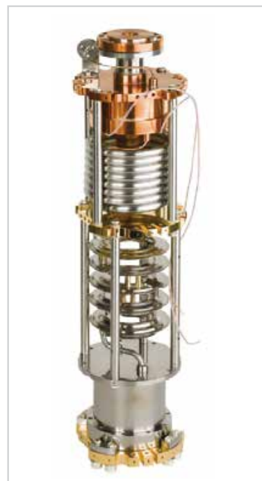
Modern dilution unit with silver heat exchanger
