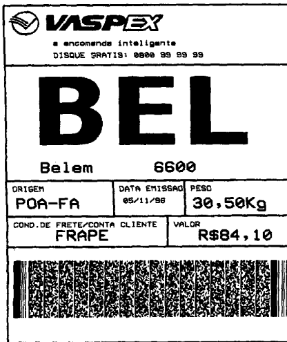
Figure 8: Shipping label from a Brazilian carrier illustrating the use of PDF417.
