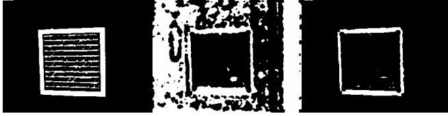
Figure 6: Left to Right: The thresholded image I_w based on whiteness, the output of texture classifier, the final mask I_x obtained by combining the two.
