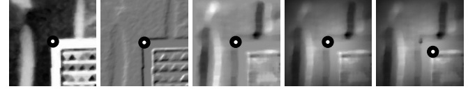
Figure 8: Left to Right: Patch extracted around marked estimated corner, gradient of the patch m respecting expected gradient directions, filtered gradient m_f , m_f weighted by a gaussian, refined location of corner.
