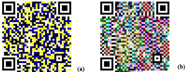
Fig. 7. Samples of the High Capacity Colored Two Dimensional Code (HCC2D) version 5 and error correction level H: 4 colors (a) and 16 colors (b) (Viewed better in color).
