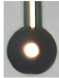
Figure 6.6: 48\mu m free air ball on 17.5\mu m wire.
