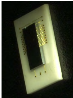
Figure 6.43: XNAP read-out chip flip-chip bonded to ceramic interposer.
