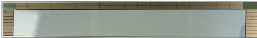
Figure 6.20: Real size photograph of the 11.9cm \times 1.6cm large silicon demonstrator assembled with 36 Switcher3 (top) and 16 DCD2 (sides) flip-chips.
