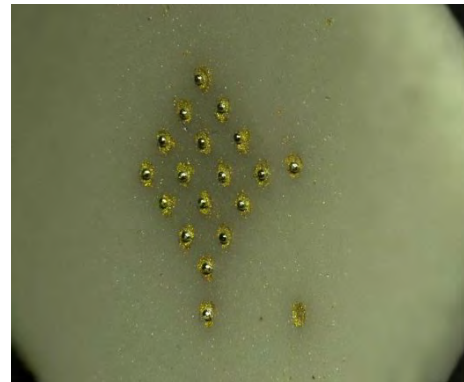
Figure 6.44: Filled through-hole vias in the ceramic interposer with solder bumps.
