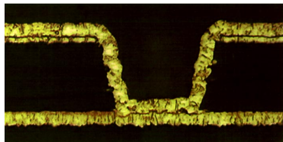
Cross Section of 6mil Laser Drilled Blind Via in FR-4
