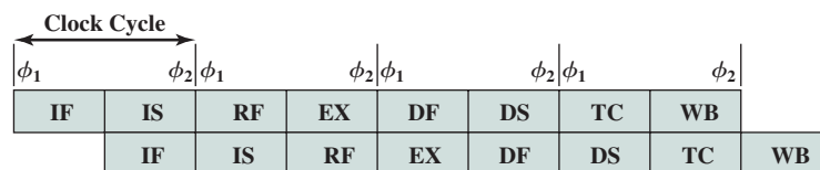
(b) R4000 pipeline
