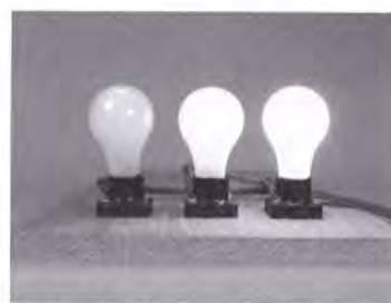
Fig. 7.3.1 As you increase the power to an incandescent lightbulb, its filament becomes hotter and emits a brighter and whiter light. The cooler filament on the left is dim and red while the hotter one on the right is bright and yellow-white. Because these bulbs are frosted, you can't see their filaments directly.
