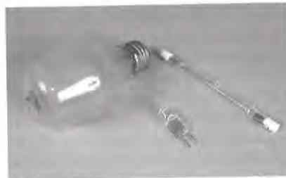
Fig. 7.3.8 These halogen bulbs operate at higher temperatures than normal incandescent bulbs and produce whiter light. The large glass envelope of the upper bulb protects a smaller lamp inside.
