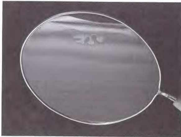
Fig. 14.1.7 Light reflected by the front and back surfaces of this soap film interferes with itself and gives the film its colorful appearance. Since the colors are determined by film thickness and since the film's thickness increases in the downward direction, the film displays horizontal bands of color.
