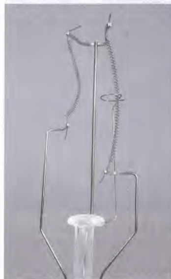
Fig. 7.3.10 The glass envelope of this three-way lightbulb has been removed to expose its two filaments. The shorter, thinner filament ( left ) uses 50 W, while the longer, thicker one ( right ) uses 100 W.
