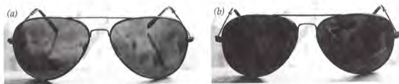
Fig. 14.1.10 (a) Ordinary sunglasses simply darken the scene. (b) Polarizing sunglasses block horizontally polarized light, the main component of glare.
