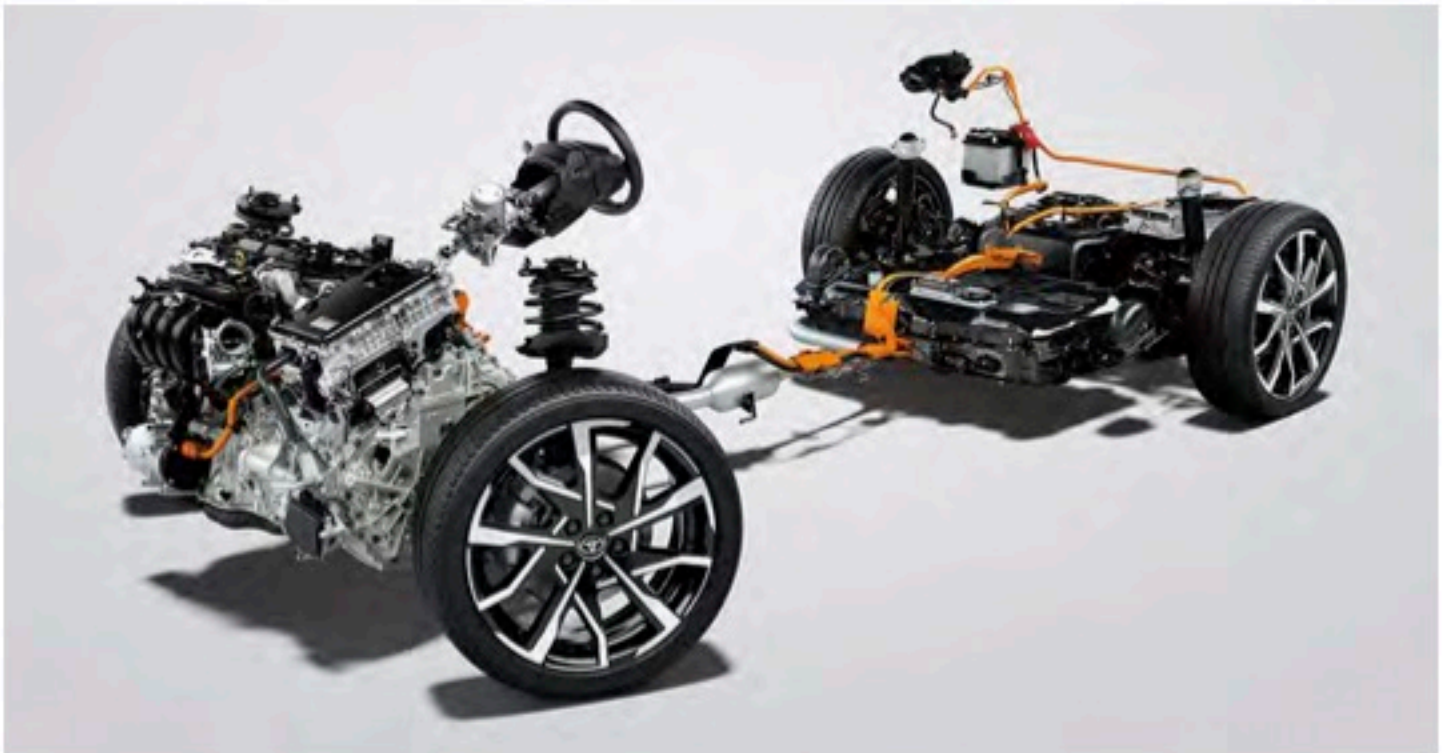
2.0-liter Plug-in Hybrid System
