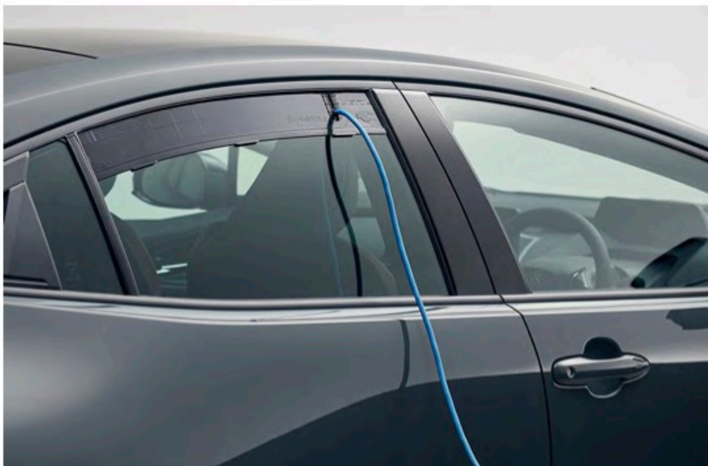
External electric power supply attachment
