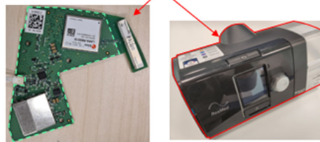
Printed circuit board, communication circuitry, and multiband antenna are arranged inside the device housing
