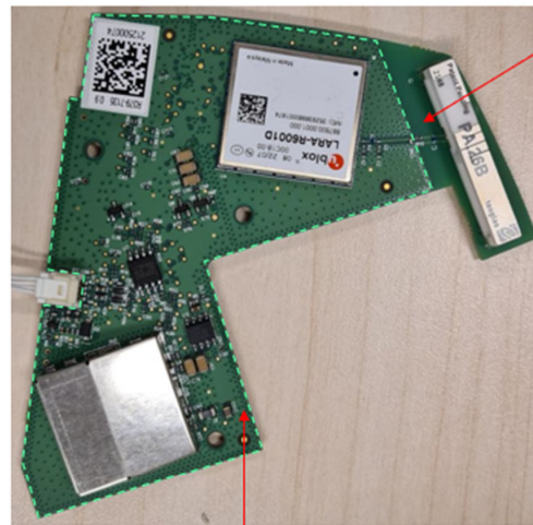
Printed circuit board comprising a ground plane layer (in dashed green)
