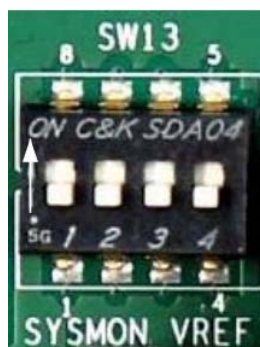
Figure 11: DIP SW13[1:4] Set to 0000
