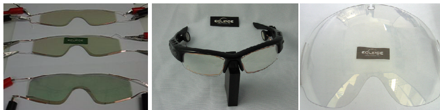
Figure 4. Representative evolution of devices from flat substrates to small curved substrates, to large curved substrates.
