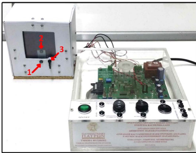
Fig. 6. Experimental set-up with the test-cell and the controller, where (1) is the external light sensor, (2) is the internal light sensor and (3) is the LED with the second internal sensor (covered during operation).
