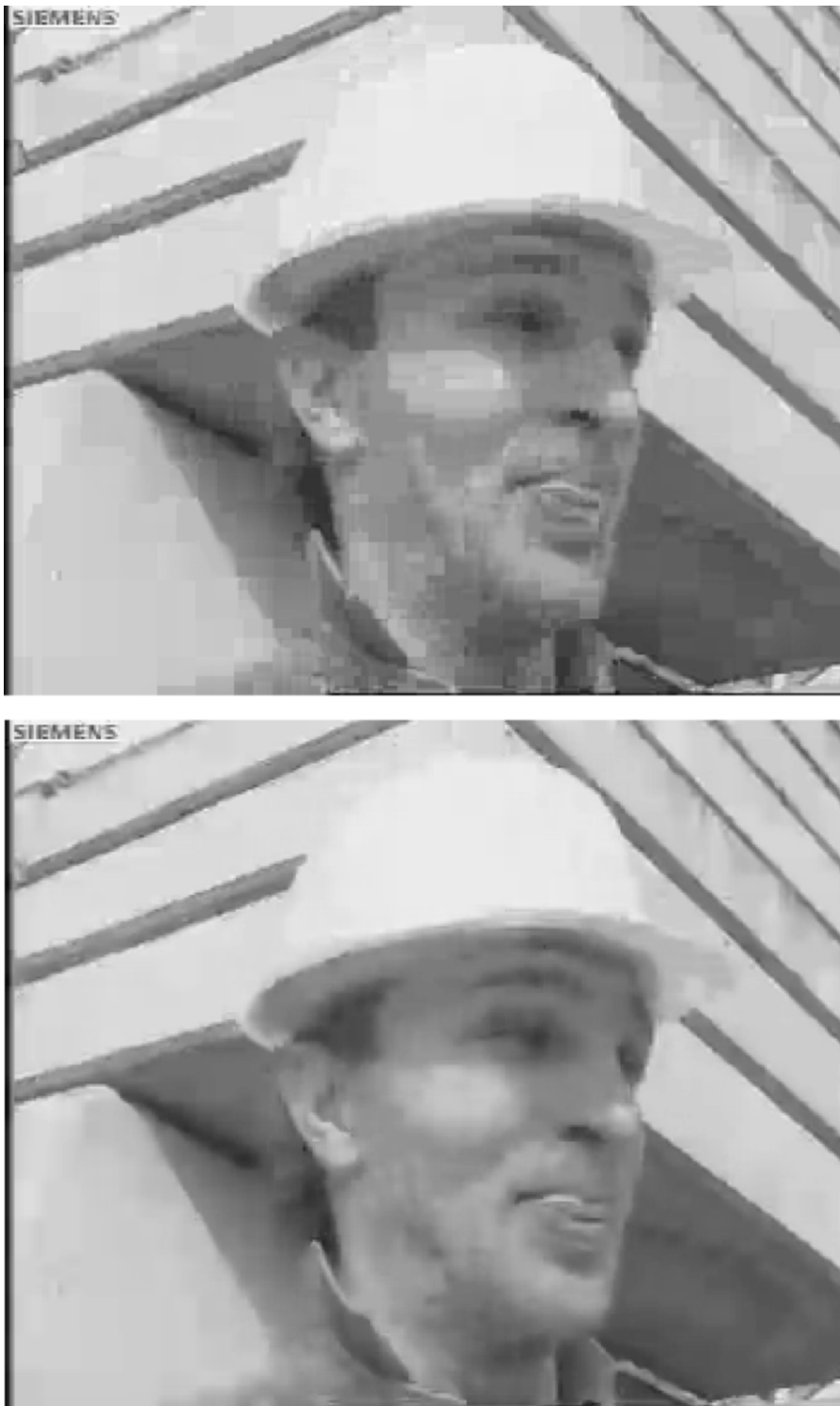
Fig. 9. Performance of the deblocking filter for highly compressed pictures. Top: without deblocking filter; bottom: with deblocking filter.
