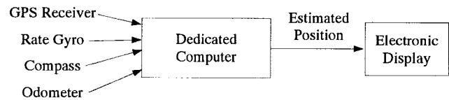
Fig. 1. Functional schematic of a land-vehicle navigation system.
