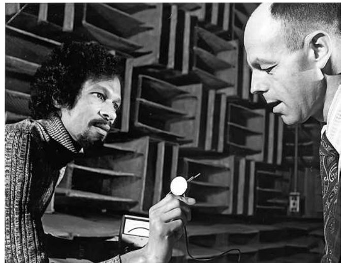
Fig 5. Photo of Jim West and Gerhard Sessler examining a second-order differential electret microphone in 1973. (Source: Bell Labs Archive)
