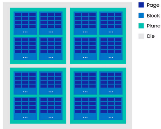
Figure 1. NAND Flash layout, illustrating a die with multiple planes, blocks and pages.
