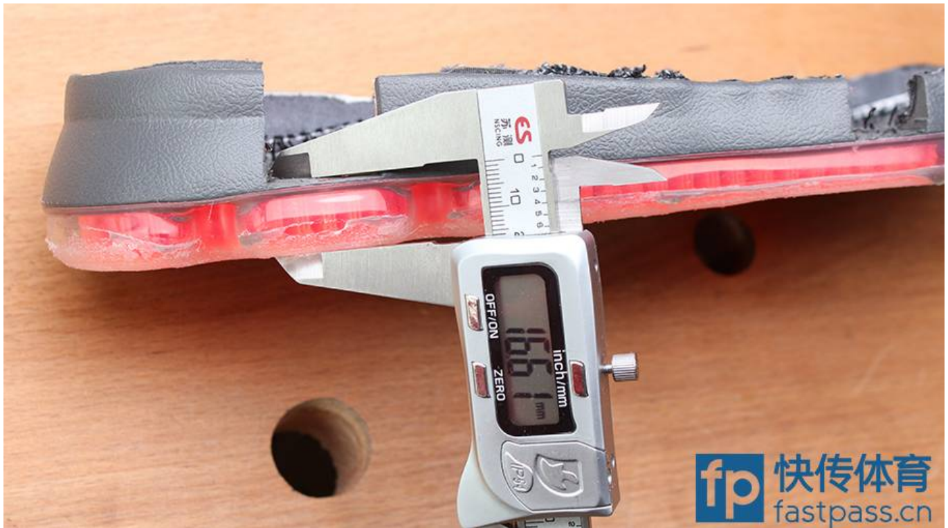
KD 9 Elite Zoom Air unit, heel area thickness
