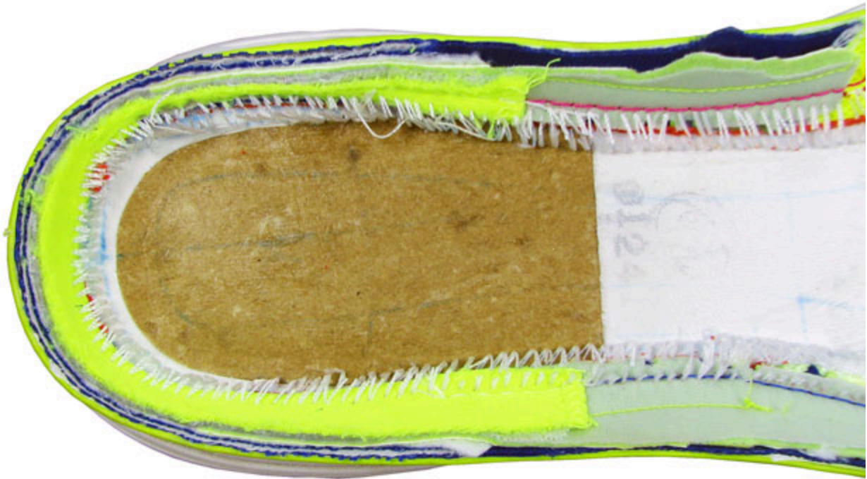
Cellulose board (cardboard) piece over the heel Zoom Air bag. This is from Vomero 8, but the Pegasus uses an identical set-up.
