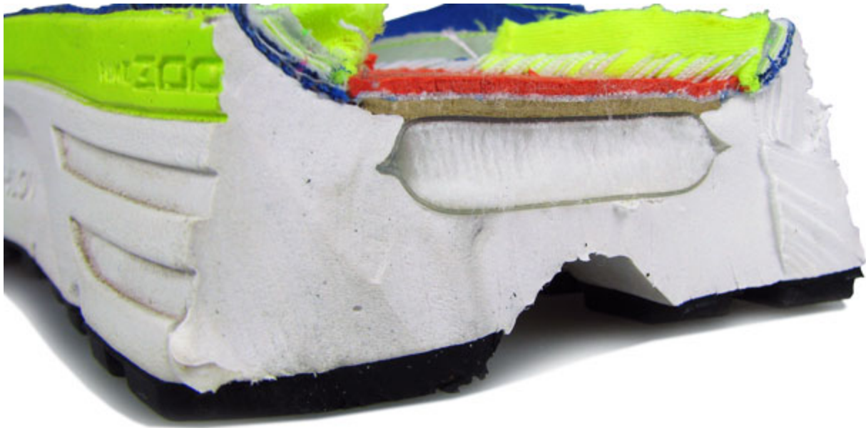
Cellulose board (cardboard) piece over the heel Zoom Air bag. This is from Vomero 8, but the Pegasus uses an identical set-up.
