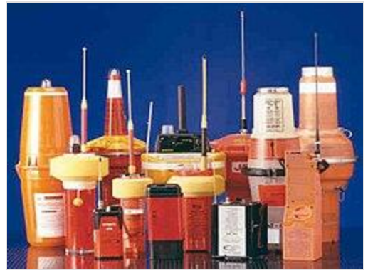
Assortment of ship emergency position-indicating radiobeacons (EPIRBs)
